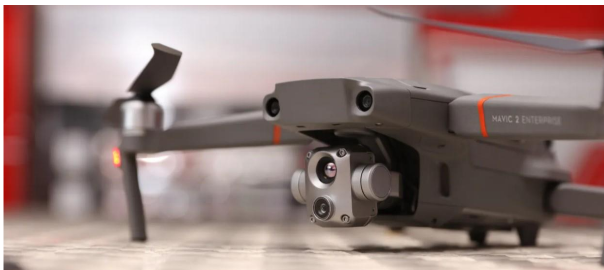
Figura 30 – Sensor Mavic 2 enterprise advanced
