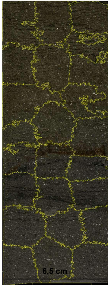
Figure 36 Example of lithology image Medium-sand_sandstone, original file: 362-u1480e-2h-2-a_shlf7853651_20160813145856.jpg, segmented by the SLIC Superpixel resulting in 26 regions. Apx: 115,07 cm 2 . Original image size: 1700 x 32007 pixels Resolution: 96 DPI. Bits intensity: 24. The grouping of pixels takes place in an appropriate way to the process, covering the entire image, separating characteristics and textures relevant to each lithology.
