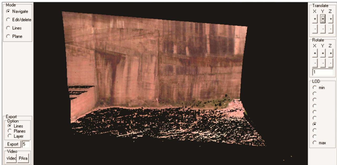
Figure 3. Outcrop Explorer's visualization and navigation module. Note the high quality of the sandstone wall as evidenced by the crossing lines (cross-stratifications) in the upper left corner of the point cloud.
