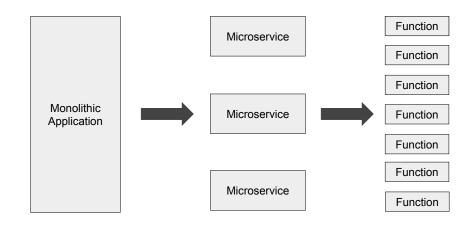
Figure 2: Comparison between monolith, microservices, and serverless functions.
