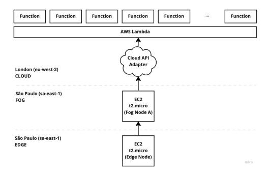
Figure 19: Architecture A with a single fog node and synchronous processing on the cloud.
