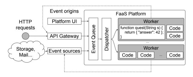
Figure 3: Main internal components of a serverless platform.
