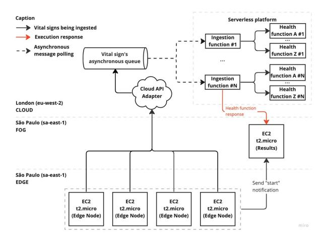
Figure 20: Architecture B without fog nodes and asynchronous processing on the cloud.
