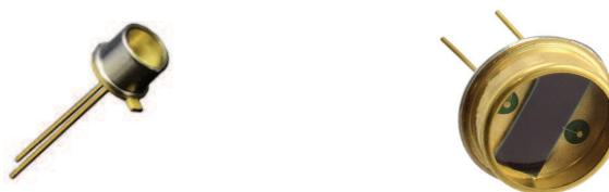
(a) emissor - MTPS8065WC    (b) fotodiodo - ODD-42WB
