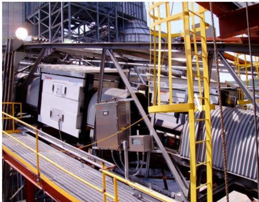
Figure 3. The online analyzer technology used in unit 4.0.
