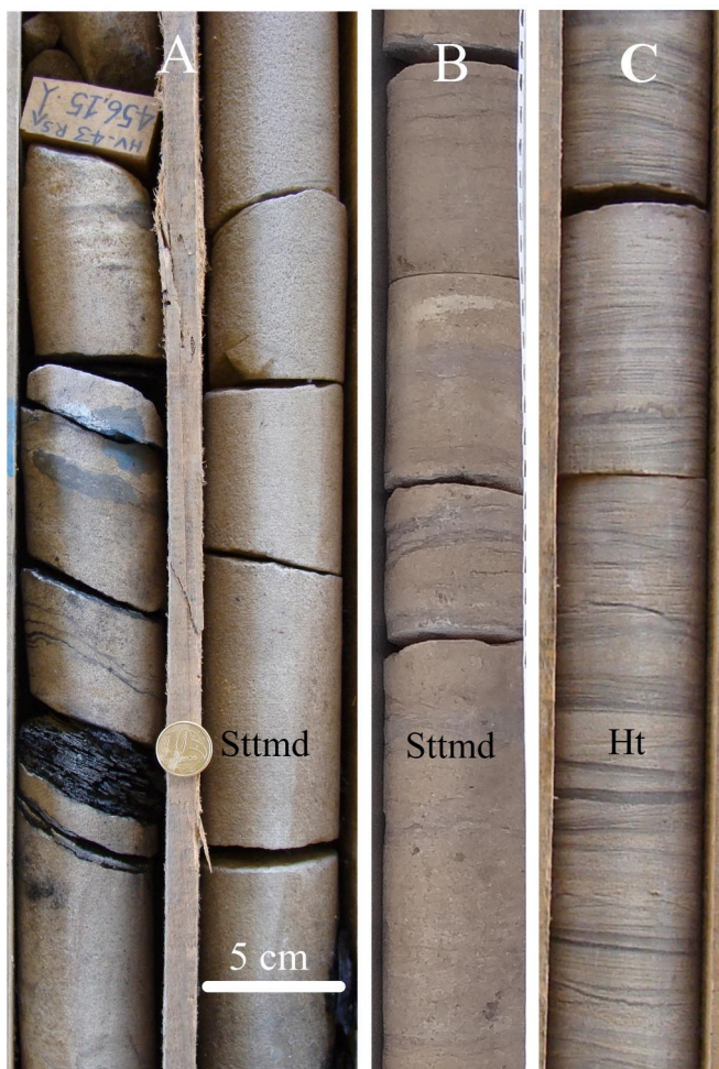
Fig. 5. Lower estuary facies association. A-B) Trough cross-bedding quartz rich sandstone with mud drapes facies (Sttmd), from core HV-43 (456.0 in the left core and 457.0 m in the right core at fig. A) and AG-01 (73 m, in fig. B). C) Heterolith facies (Ht) from core AG-01, at 91 m depth.
