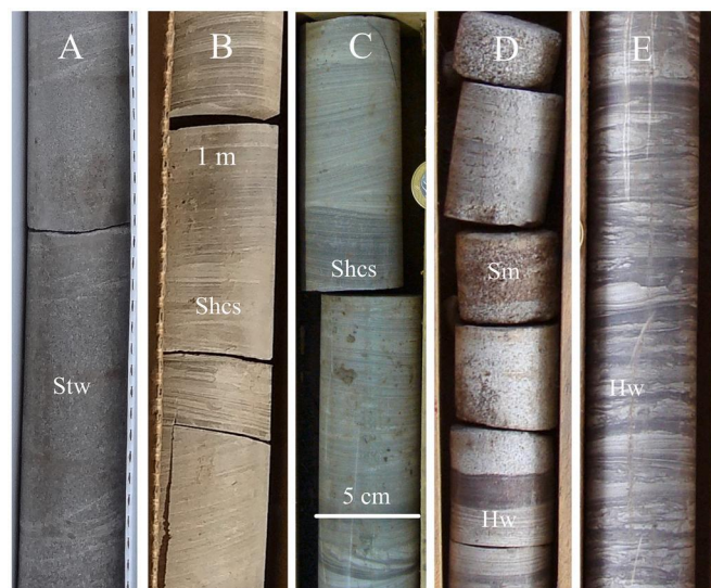
Fig. 8. Barrier facies association. A) Trough cross-bedding quartz rich sandstone facies (Stw) in core HN-59, at 328 m depth. B–C) Hummocky cross-stratification sandstone facies (Shcs) in core HV-45 (at 171 m depth, in fig. B) and SC-109 (at 65 m depth, in fig. C). D) Bioturbated heterolith facies (Hw) and massive sandstone facies (Sm) in core HV-45, at 156 m depth. E) Bioturbated heterolith facies (Hw) in core HV-45, at 158 m depth.
