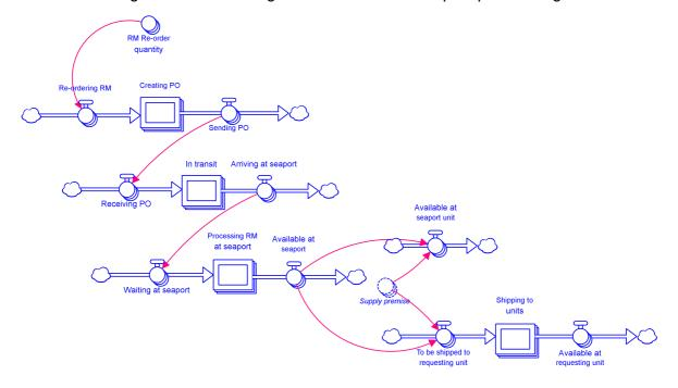
Figure 28 – Ordering raw material and seaport processing
